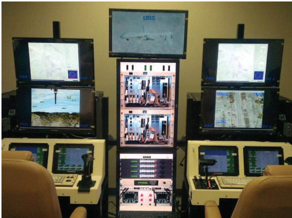
Figure 1. X-TUAS™ simulators in the full crew (pilot and sensor operator) station configuration (Source: http://www.urs-simulation.com ).
