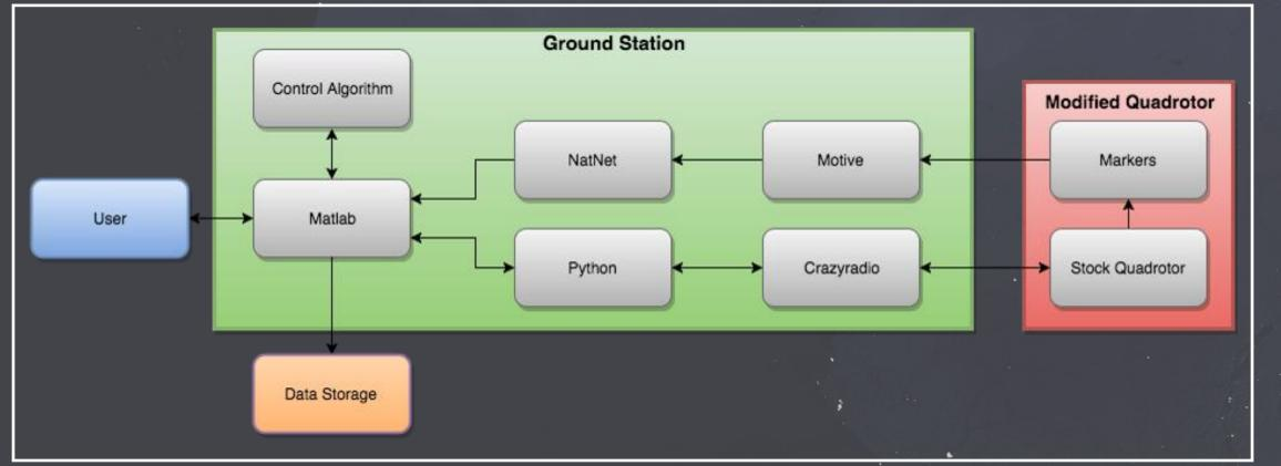
The diagram above is a high-level, technical representation of the communication pathways present in the system. It should be noted that the input and output with the modified quadrotors is completely automated.
