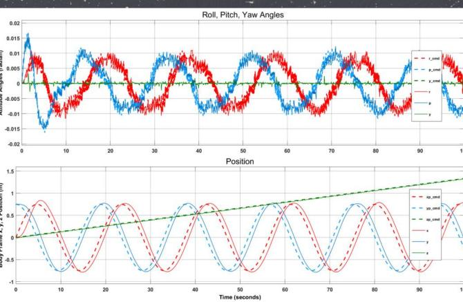
Additionally, the results show that a refresh rate of 10 Hz (*left*) is necessary for reasonable agent performance. This realization confirms that the developed system will meet the needs; the measured refresh rate is approximately 30 Hz (*right*).
