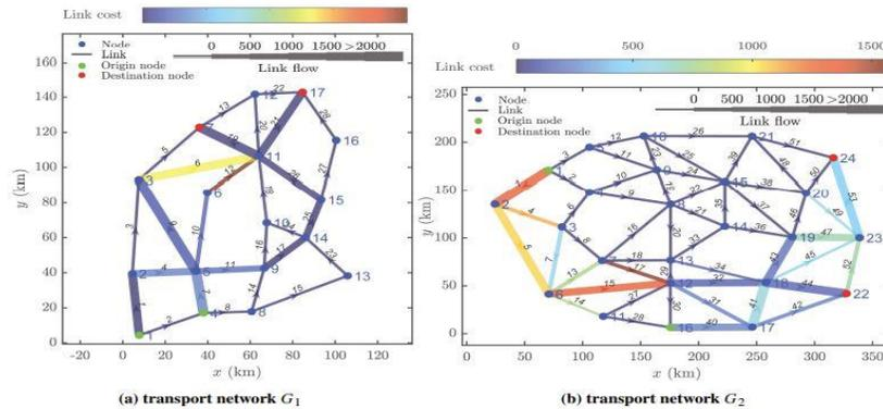
Fig. 14 Traffic assignment result for the whole network in terms of flow allocation and link cost
