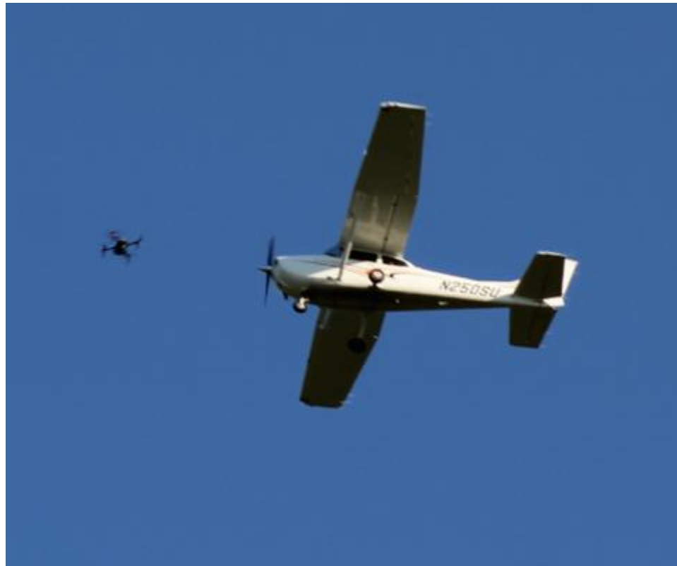
Figure 9. Ground observer image of Participant 2, Intercept 3. Participant 2 indicated that the sUAS appeared to be at a greater altitude than the aircraft. Small UAS and aircraft altitudes were fixed at 400 feet AGL and 600 feet AGL, respectively.
