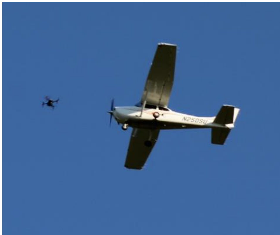
Figure 9. Ground observer image of Participant 2, Intercept 3. Participant 2 indicated that the sUAS appeared to be at a greater altitude than the aircraft. Small UAS and aircraft altitudes were fixed at 400 feet AGL and 600 feet AGL, respectively.
