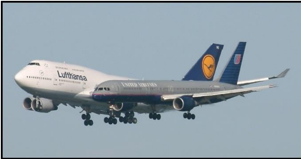
Figure 8. Optical illusion of Lufthansa 747-400 and United Airlines 757-200 on simultaneous approaches to runways 28L and 28R at San Francisco (SFO). The distance offset is difficult to perceive, as there is a natural tendency to relate objects in terms of comparable relative size. In this case, however, the 747-400 is substantially larger than the 757-200, which is not apparent by visual comparison alone. This figure illustrates a similar optical illusion to that encountered by experimental participants in which size differential adversely affected observers’ ability to accurately judge distances. Used with permission, courtesy of photographer Ben Wang, Airliners.net .
