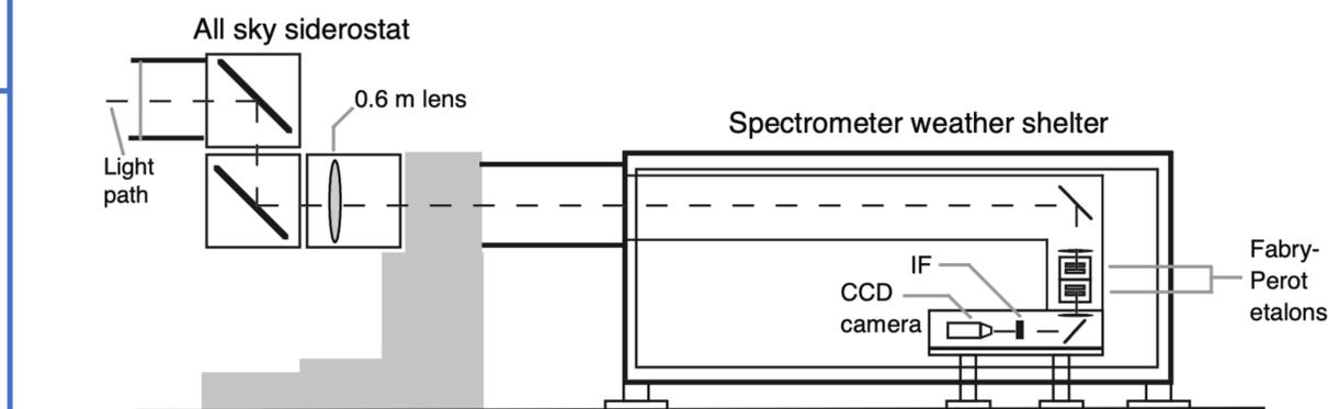
A schematic of the WHAM instrument. The dashed line denotes the path of an on-axis ray through the system. As shown in the diagram, both flat mirrors in the siderostat rotate independently, allowing all-sky pointing and tracking.
