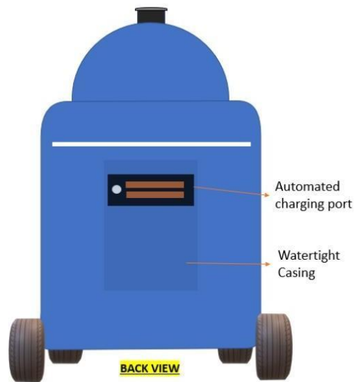
Figure 6: Back View of Bobo Robot
