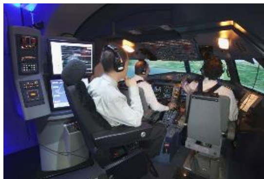
Figure 5. ATR 600 Flight Simulator with Instructor Station. (Retrieved from http://www.ainonline.com/sites/default/files/uploads/2014/02/500-ain-sing-atr-training-sim-in-singapore-1.jpg . Courtesy of AIN. Reprinted with permission.)
