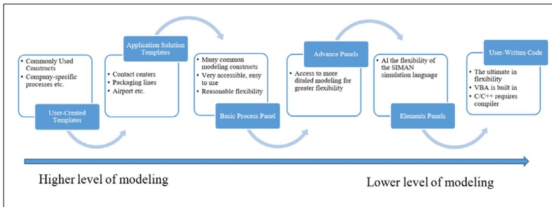
*Figure 1.* ARENA's Hierarchical Structure. *Note.* Adapted from *Simulation with Arena* by W. D. Kelton, R. P. Sadowski, & N. B. Swets, 2010, New York, NY: McGraw-Hill Companies, Inc. Copyright 2010 by the McGraw-Hill Companies, Inc.
