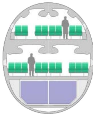
*Figure 4.* The A380 cabin cross section with economy class seating. Retrieved from Airbus A380 seat configurations in *Wikipedia, n.d.*, Retrieved October 21, 2015, from [https://en.wikipedia.org/wiki/Airbus\\_A380\\_seat\\_configurations](https://en.wikipedia.org/wiki/Airbus_A380_seat_configurations).
