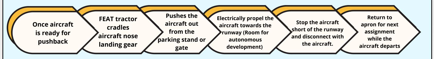
• During the towing process, the pilot retains the capability to maintain control over the taxiing operation, allowing for immediate intervention should the taxibot exhibit unexpected behavior, thereby ensuring safety. As automation technology in aviation continues to advance in reliability, there is potential for the entire taxiing operation to shift towards full autonomy, effectively reducing the workload of the pilot.
