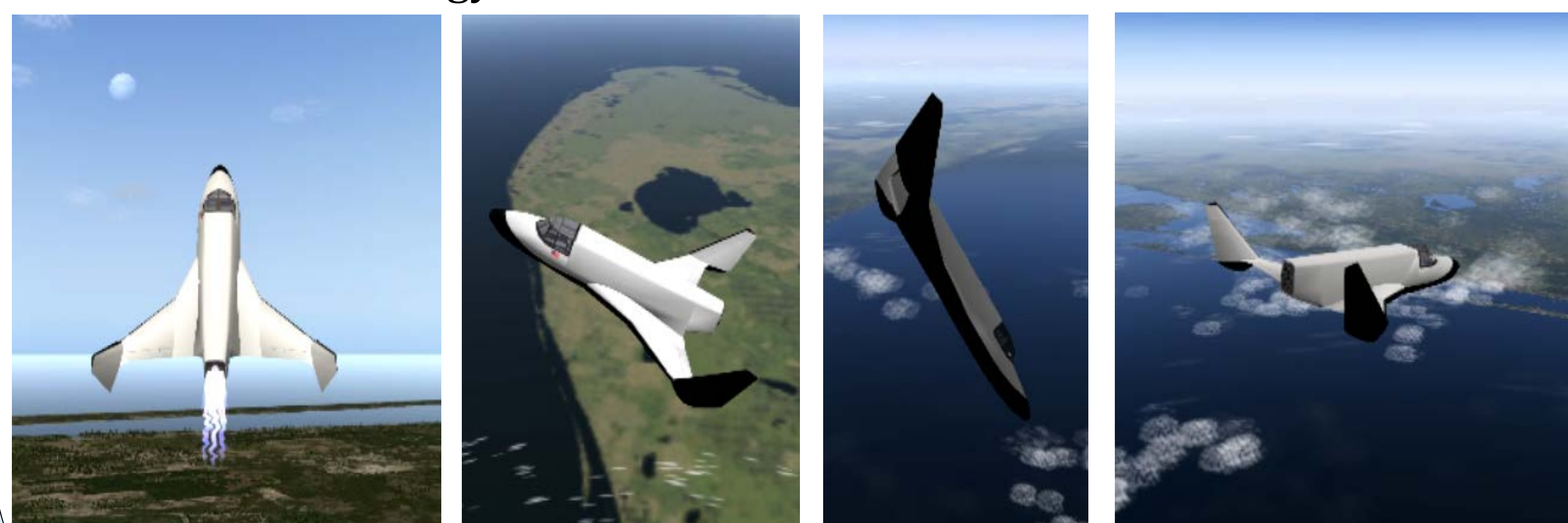
a: Takeoff b: Pitch-up c: Nose down d: Glide
