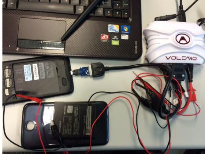
Picture 1. Cable connection using Volcano Box
