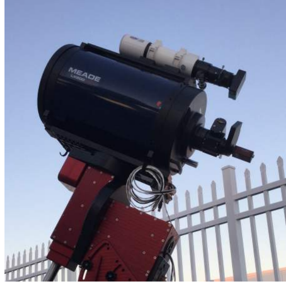
(b) Meade LX200 and Borg 77EDII in optical feedback track mode.
