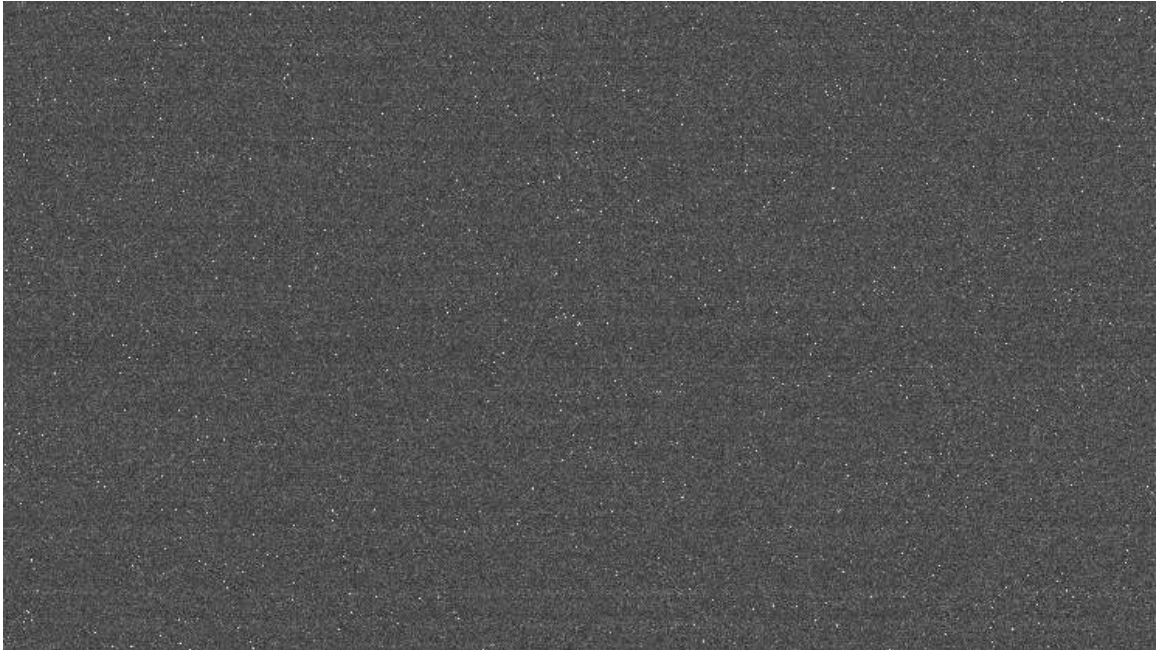
Figure 5.1: A crop from a master dark frame created by averaging fifty 150 ms darks from the Manta G-235 CMOS detector.
