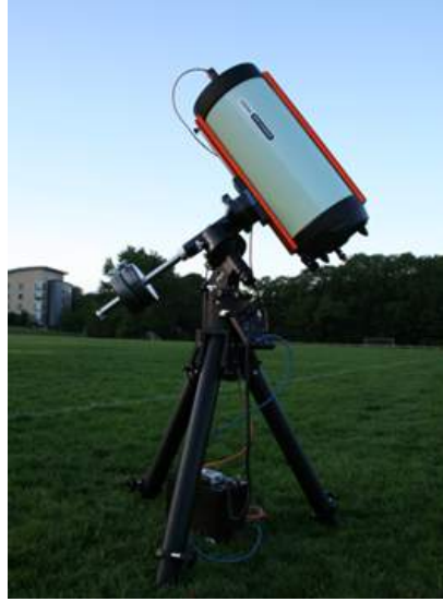
Figure 1.4: The Celestron RASA deployed in the field on an amateur astronomy mount is capable of observing CubeSat sized objects.
