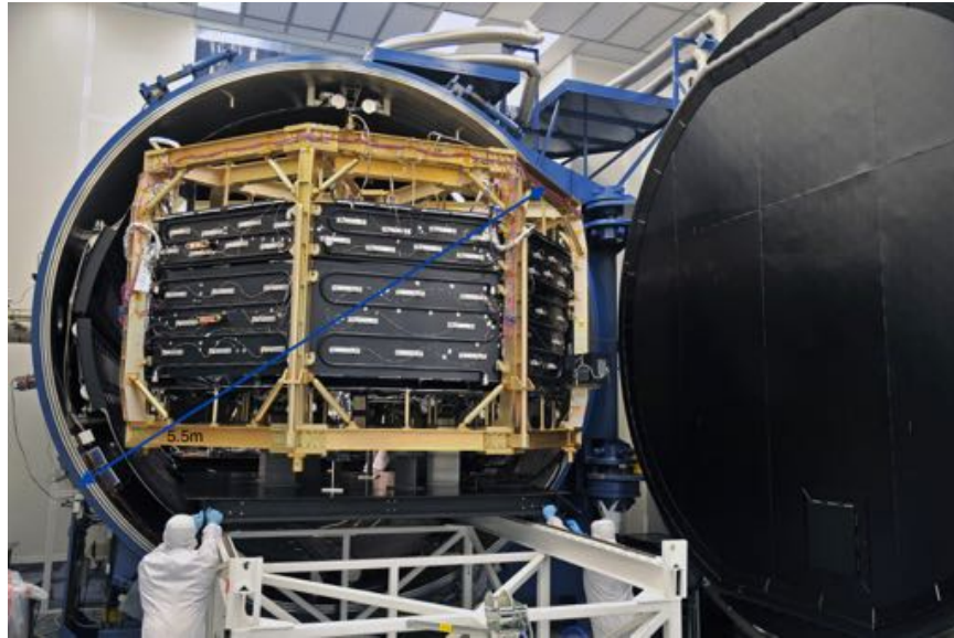
Figure 2.4. The first MMS mission satellite being put into the thermal vacuum test chamber at the NRL Thermal Fabrication and Test Facility (Parry, 2014)
