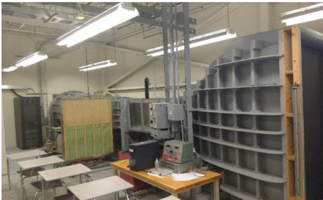
Figure 3.39 Open loop windtunnel (author).
