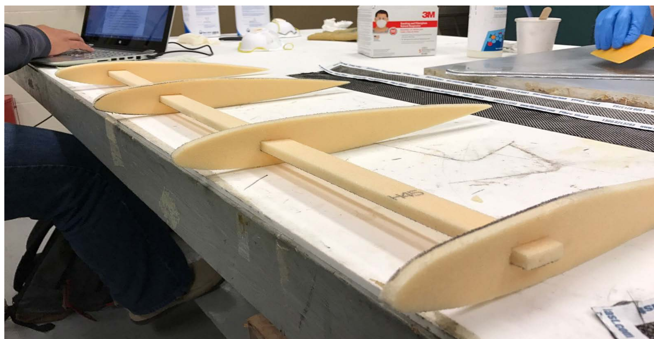
Figure 1. Main Wing Skeleton Structure (1 spar with 4 ribs)
