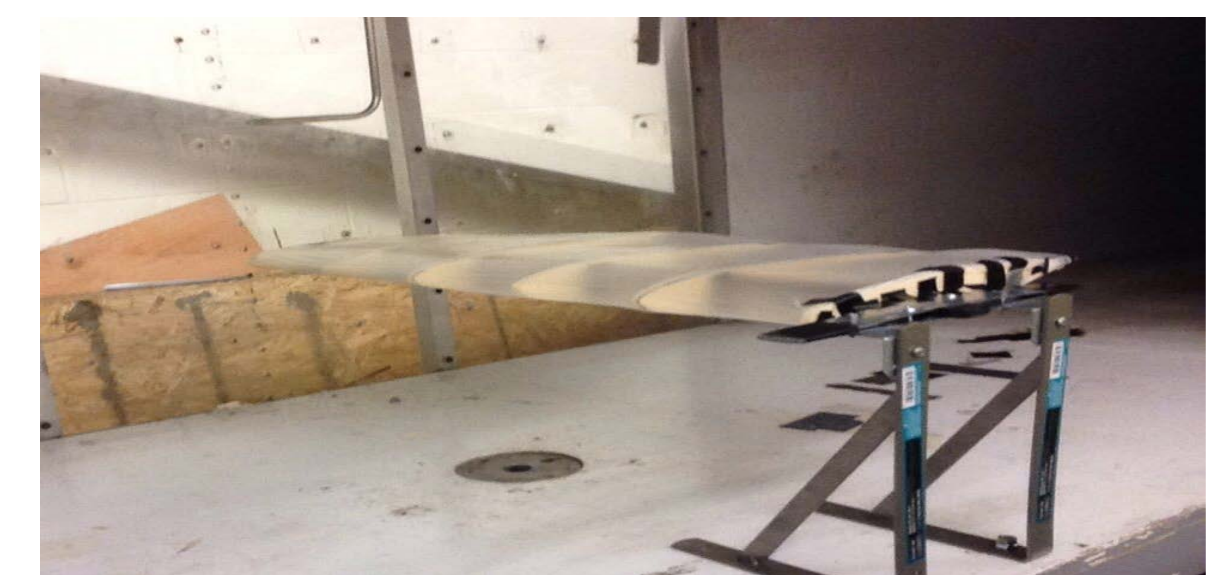
Figure 5. Main Wing Configuration in the Wind Tunnel
