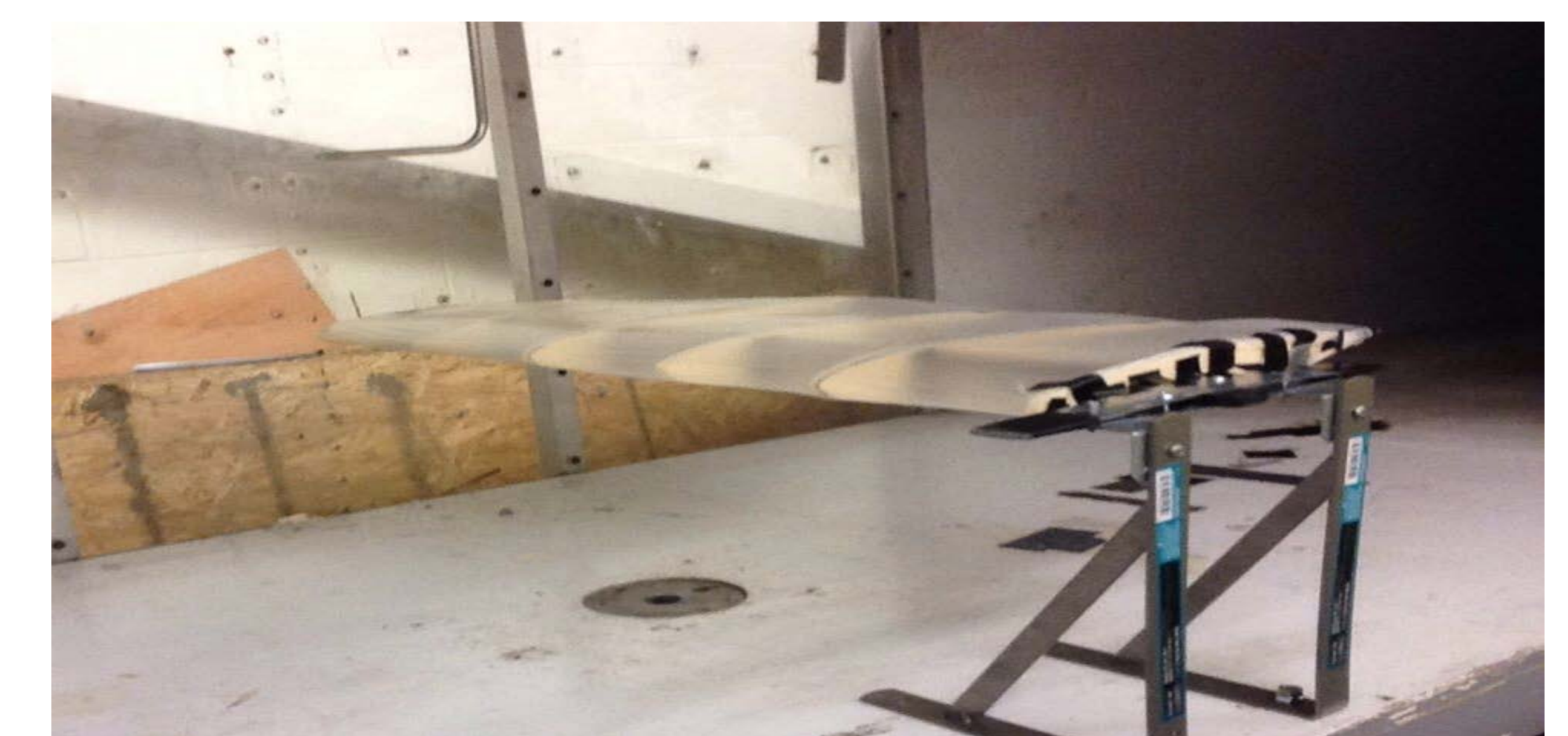
Figure 5. Main Wing Configuration in the Wind Tunnel
