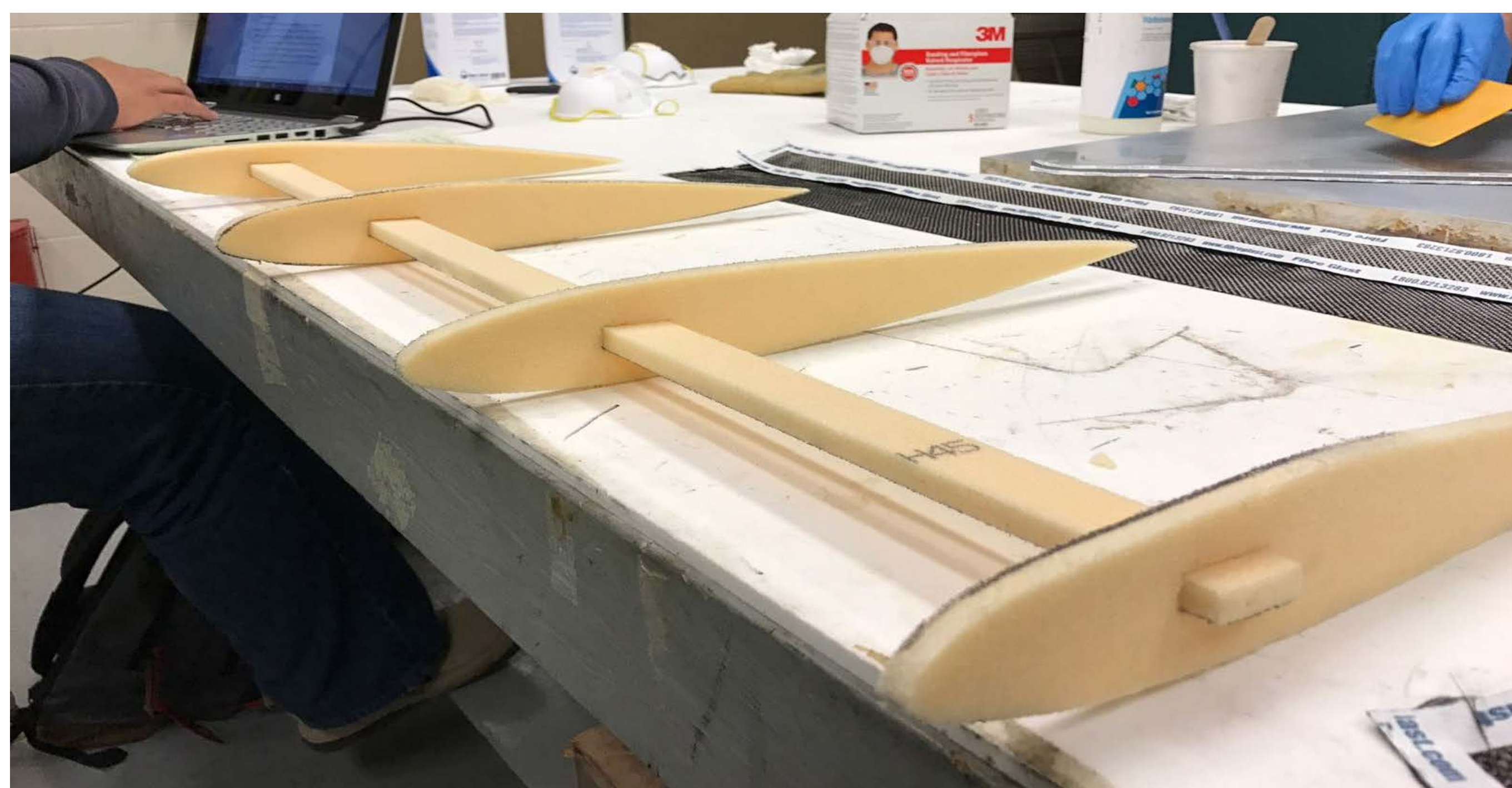
Figure 1. Main Wing Skeleton Structure (1 spar with 4 ribs)
