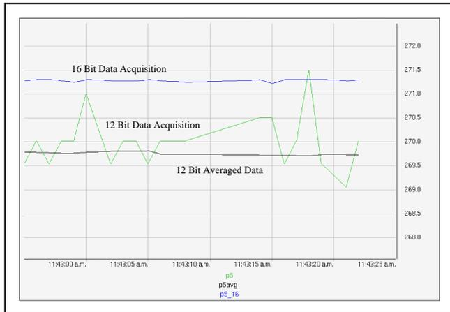
Figure 2 12-bit vs 16-bit Data Acquisition System
