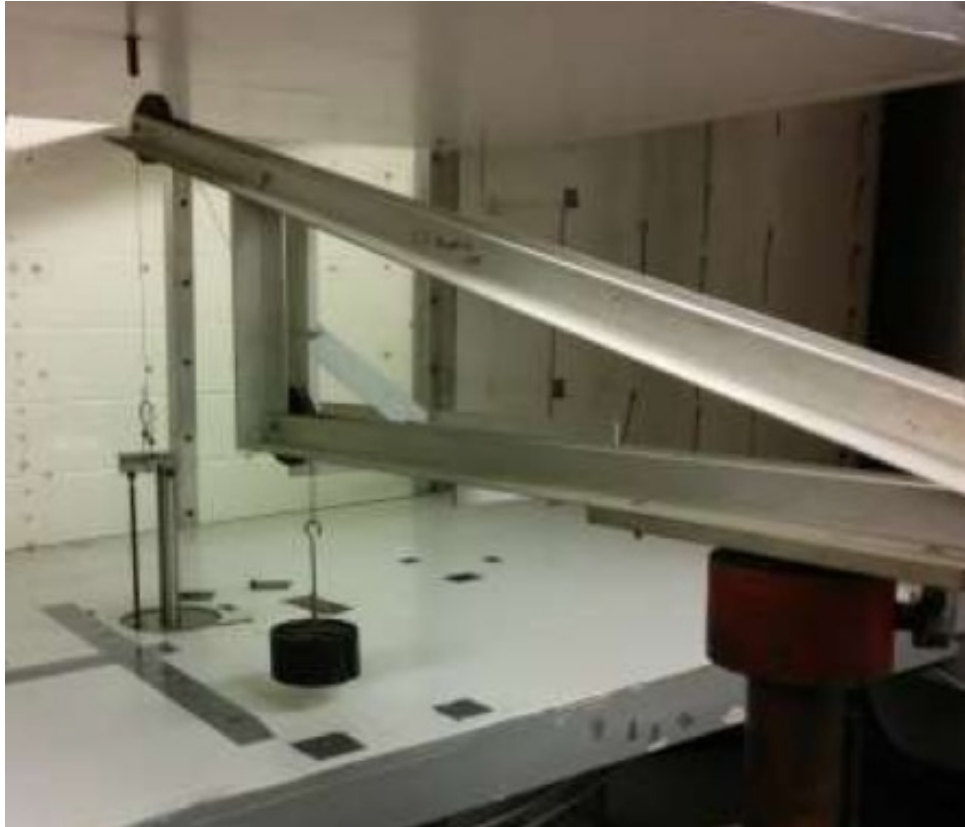
Figure 5.2.. Lift component calibration
