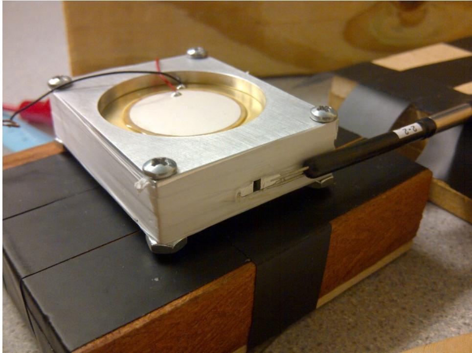
Figure 4.7.. Hot wire probe and Model-R SJA with rectangular slot
