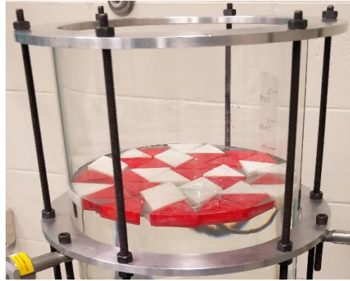
Figure 1.6 Reconstructed floating Magnetoactive Micro-Baffles setup
