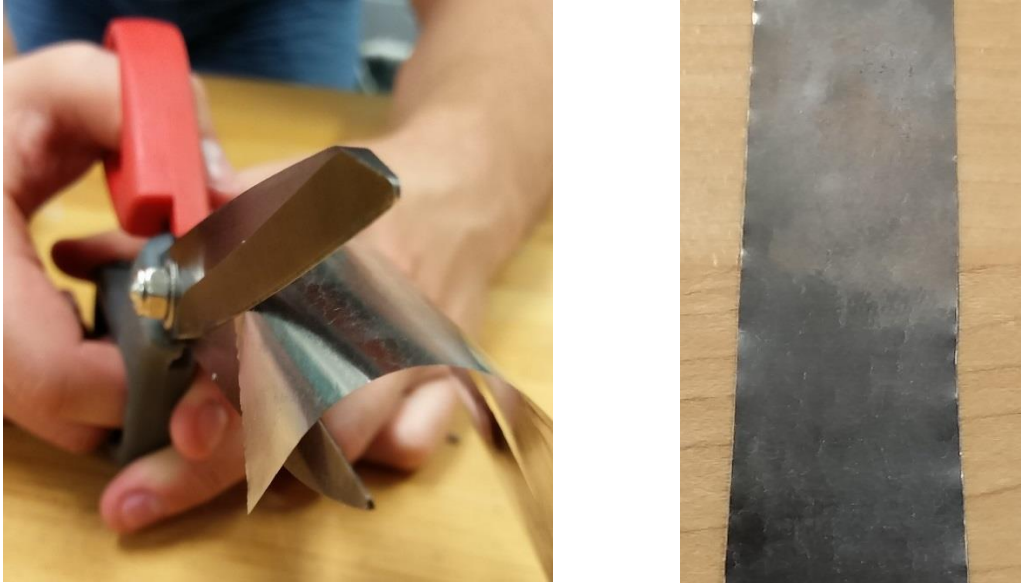
Figure 3.3 Metglas 2605SA1 sheet bending under scissor cutting edges (left) and final cut with straight edges (right)
