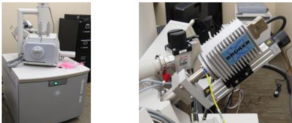
Figure 3.1 Scanning Electron Microscope FEI™ Quanta 650 present in Embry-Riddle Aeronautical University. SEM setup (left) and EDX setup (right)
