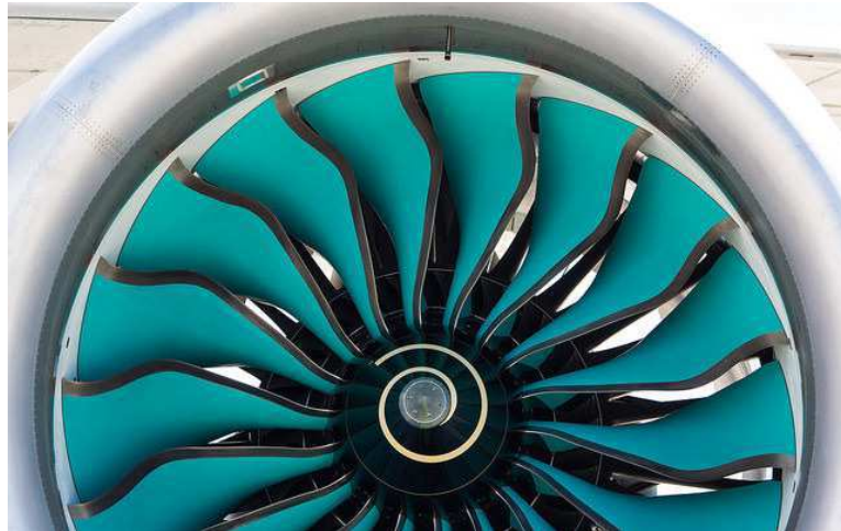
Figure 1.5 Example of a modern transonic fan showing 3D features (Rolls-Royce plc, 2014).
