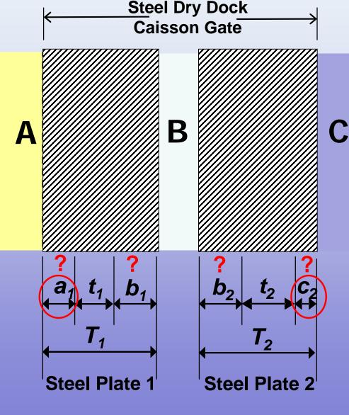
$T_1 = a_1 + t_1 + b_1$  $T_2 = b_2 + t_2 + c_2$ But if  $b_1 \approx b_2$  then...  $b_1 \approx b_2 = T_1 - t_1 - a_1$  $= T_2 - t_2 - c_2$  $T_1 - T_2 = a_1 - c_2 + t_1 - t_2$ Material loss relationship:  $a_1 = f(c_2)$  $a_1 = c_2 + T_1 - T_2 + t_2 - t_1$ **Constants Random** Variables for *a*₁ ≥ 0
