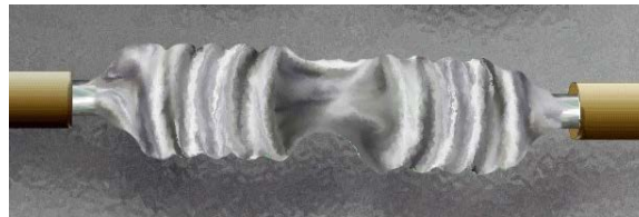
Figure 18: Soldered Western Union
