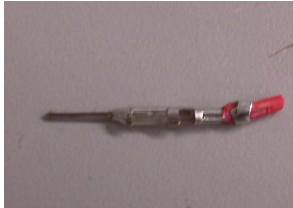
Figure 58: Lack of Conductor in Crimp
