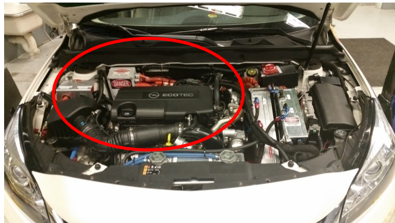
Figure 5: Diesel Generator in Engine Bay
