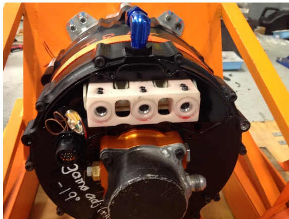
Figure 71: Traction Motor with Gland Plate Removed
