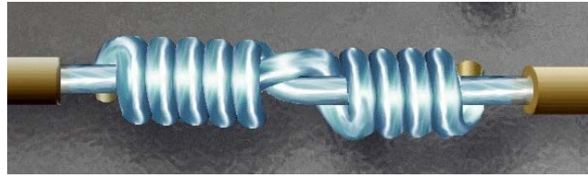
Figure 17: Completed Wrap for Western Union
