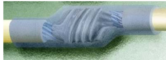
Figure 15: Heat Shirked Connection
