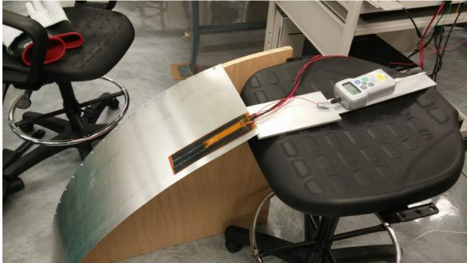
Figure 6.11. Test Setup to Determine Adhesion with MFC Use
