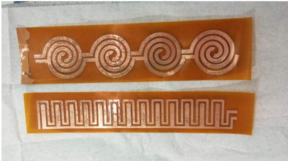
Figure 5.6. Completely Etched Pads with Exposed Electrode Designs
