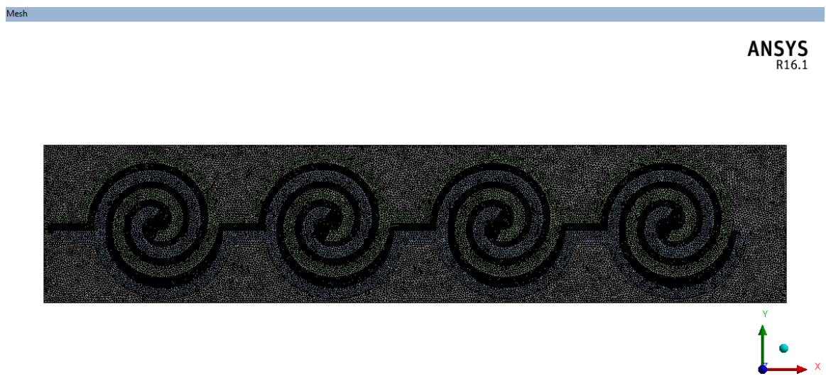
Figure A.3. Mesh Density on LF9120 Spiral Model
