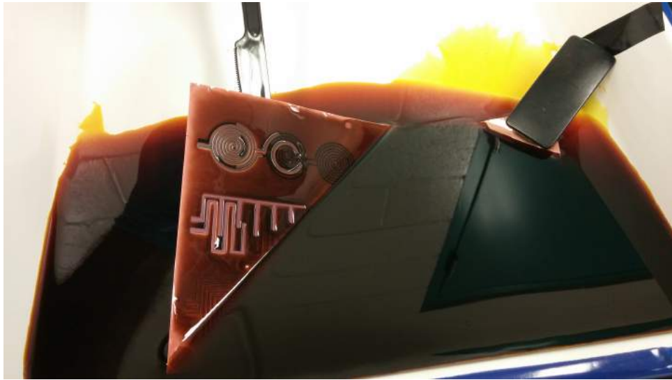
Figure 5.4. Pyralux Pads Submerged in Ferric Chloride
