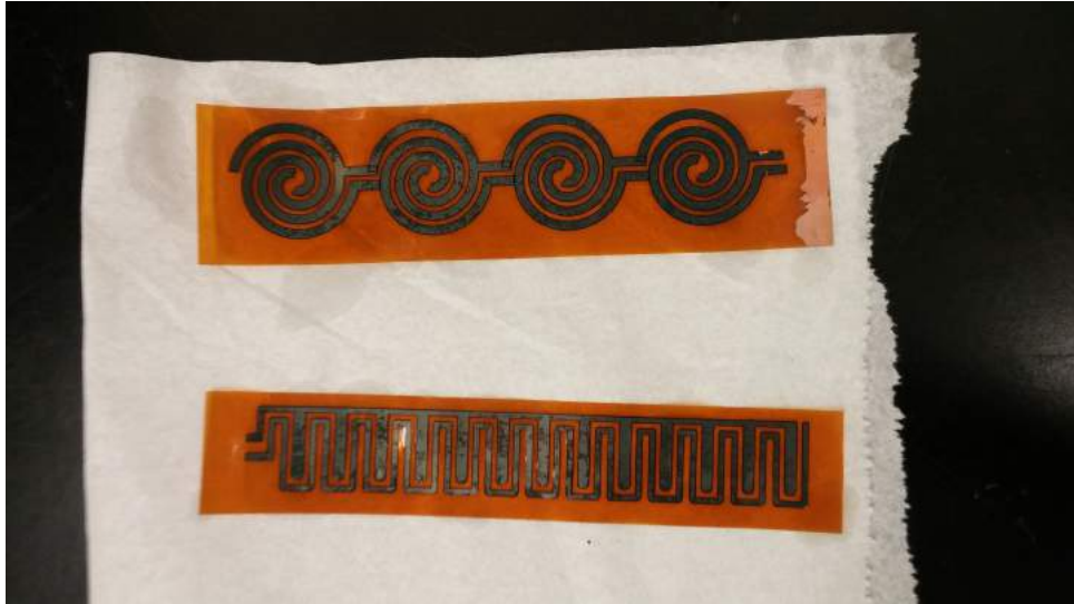
Figure 5.5. Etched Pads With Remaining Wax Layer
