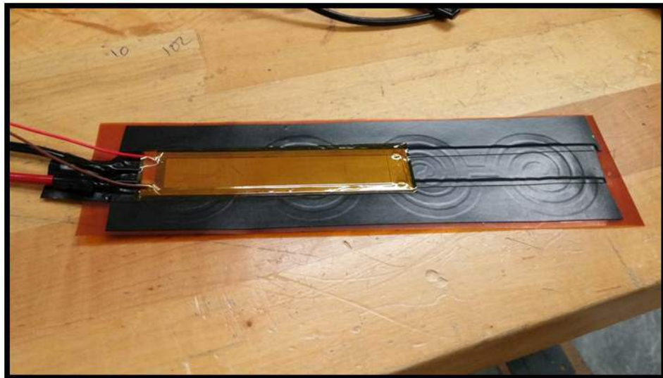
Figure 5.8. Spiral Pad with attached MFC actuator
