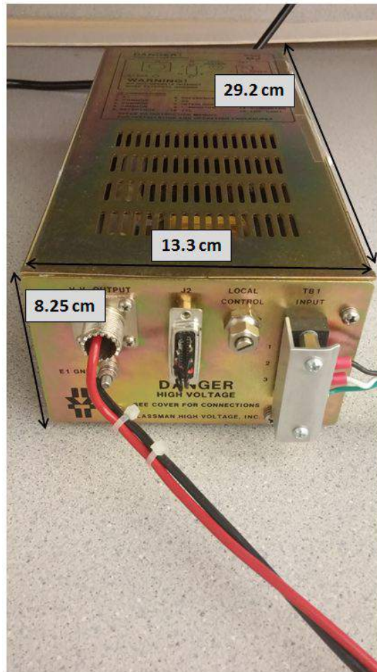
Figure 6.2. Glassman MJ3P5000 3kV Power Supply
