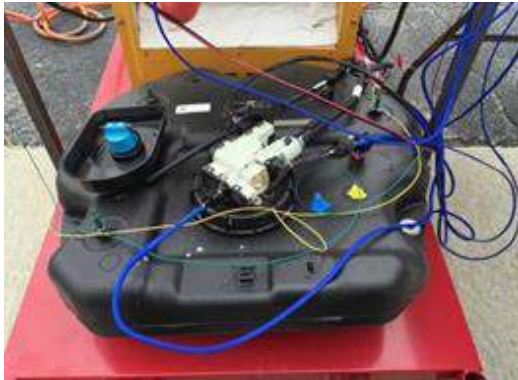
Figure 4.4.: Diesel Exhaust Fluid Tank
