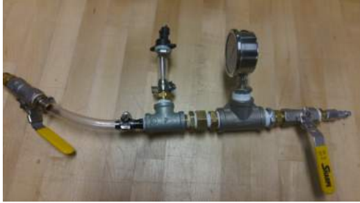
Figure 4.5.: Pressure Sensor Calibration Setup
