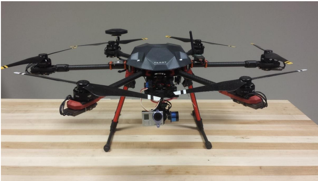
Figure 5. An example of a UAV with a gimbal mounted camera. This particular UAV is carrying a GoPro Hero3+ camera.
