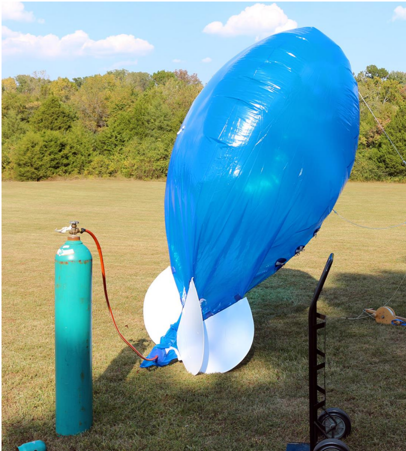
Figure 4. An example of a helium blimp being inflated before flight. When full, this particular blimp is thirteen feet in length (just under four meters) and holds approximately 300 cubic feet of helium (eight and a half cubic meters).
