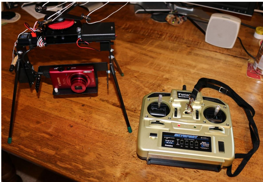
Figure 6. An example of a customized kit-built remote camera rig carrying a Canon PowerShot ELPH 130IS for use with tethered platforms.
