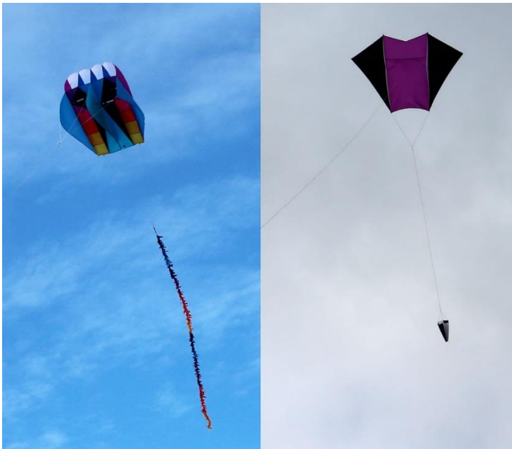
Figure 3. Two examples of tethered kites. The kite on the left is a soft kite that can fly in winds between 5 and 30 mph, although higher speeds of 15mph or more are necessary to lift a camera rig. The kite on the right is a rigid kite that has carbon fiber spars to add support. This allows the kite to fly and lift a camera rig in lower windspeeds of around 10 miles per hour or more. Higher windspeeds of 20mph or more can damage the carbon fiber spars.
