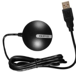
Figure 2.2 GlobalSat BU-353 GPS receiver
