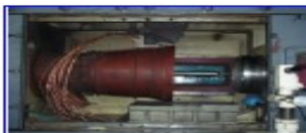
Figure 1.5. Test model installed in hypersonic wind tunnel in CAAA (Liu and Jiang, 2013).
