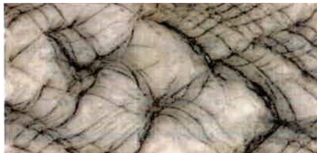
Figure 2.9 Experimental soot foil pattern for an unstable detonation wave
