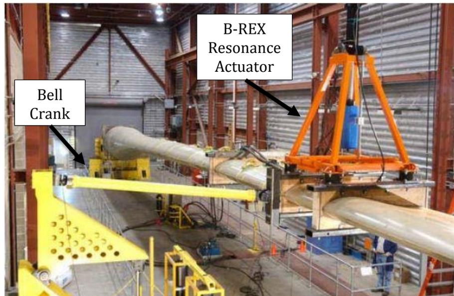
Figure 2.4: B-REX Test Set-up
