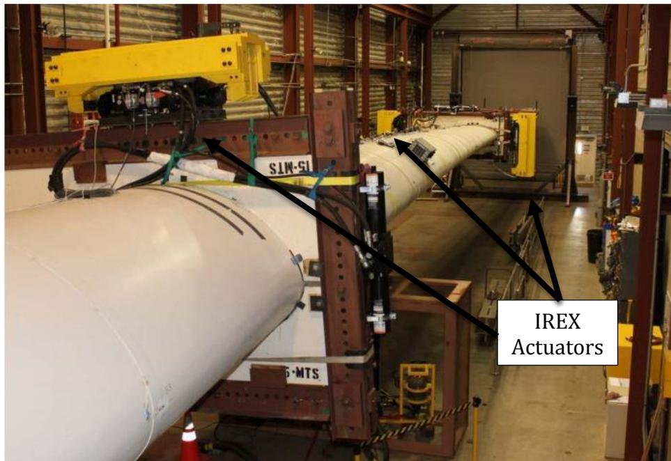
Figure 2.5: Quantum Resonance Test Set-Up
