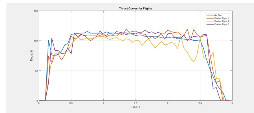
Figure 5. Plot comparing the thrust curves from all flights thus far.
