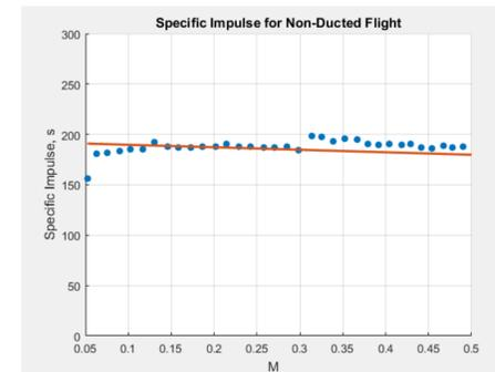
Figure 3. Plot showing the vehicle's near constant specific impulse without the duct attached.
