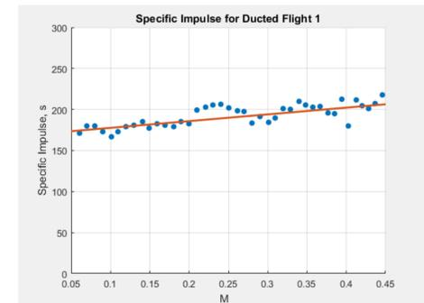
Figure 4. Plot showing increase in ISP during ascent.
