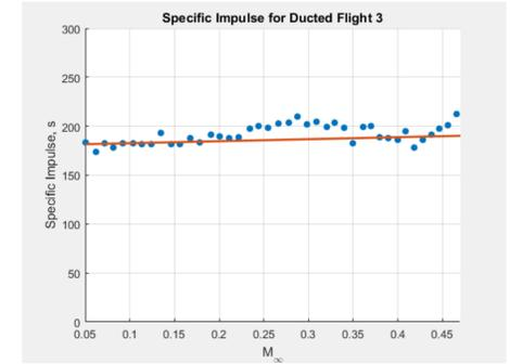
Figure 6. Data from most recent ducted flight showing very slight increase in ISP.
