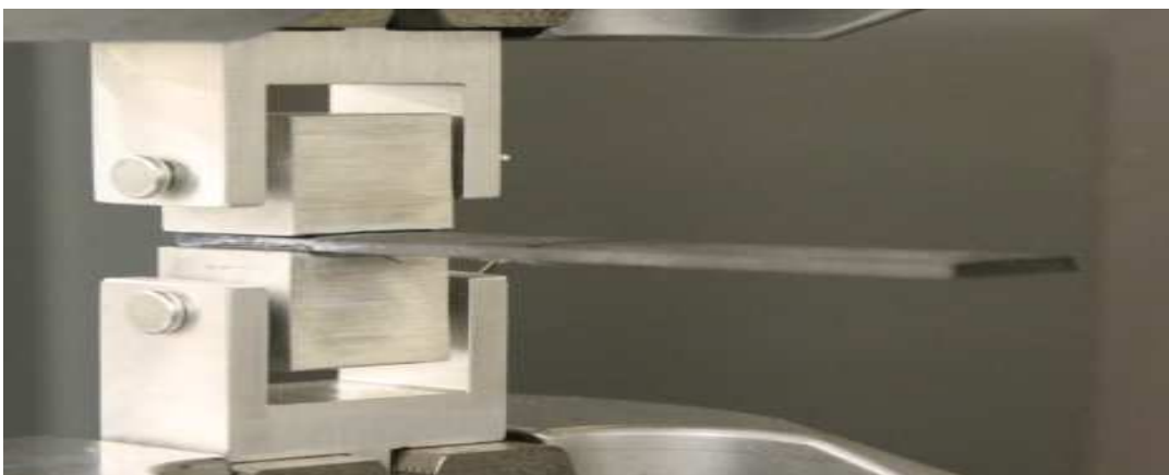
Figure 5.1b. DCB test configuration for fracture and fatigue characterization.
