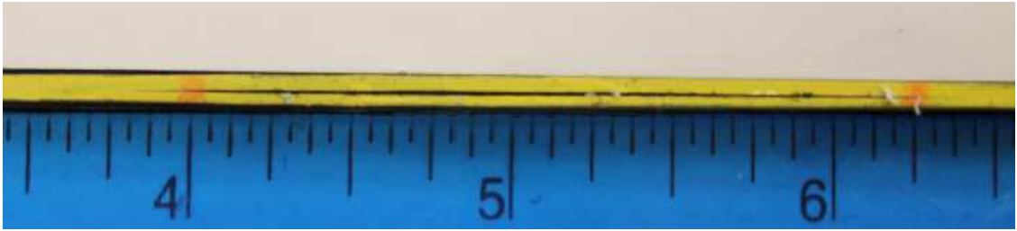
Figure 6.9 Delaminated Specimen Using Visual Measurement.
