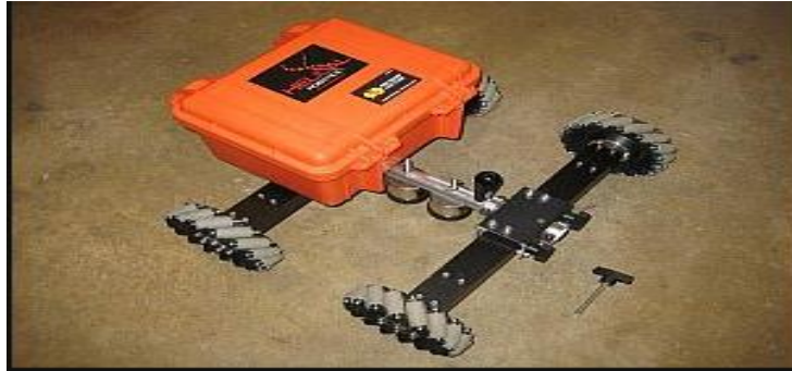
Figure 1.1: Mecanum Wheels Mounted on Robot Manufactured by Helical Robotics [2]
