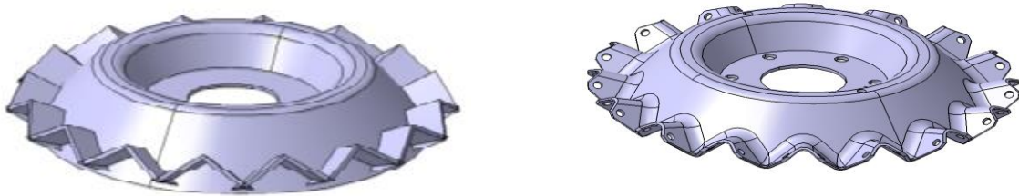
Figure 3.1: Plate Concept 1 Designed in CATIA & AndyMark Wheel Design [3]
