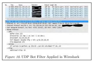
In Figure 10 above, packets have been filtered only to show port 53413 packets, which are displayed as being of the "UDP Bot" Protocol type. Packet 10 is decoded showing a tree entry for
