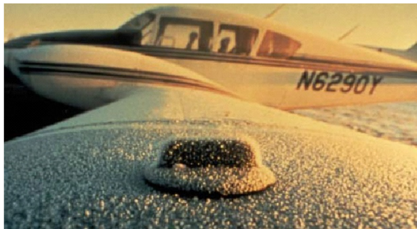
Figure 3. Ice formation on aircraft wing structure (Steuernagle, Roy, & Wright, 2002)
