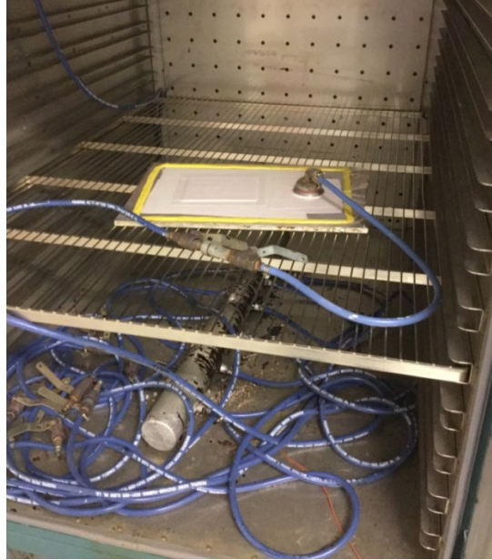
Figure 27. Vacuum compressed proto types in 260 degree oven
