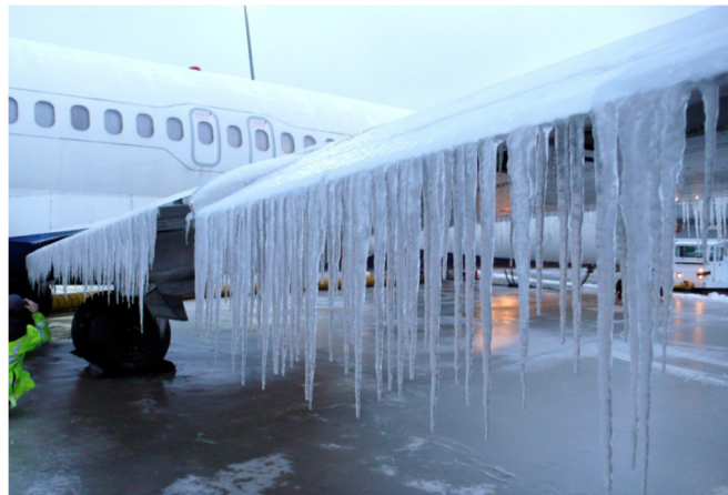
Figure 4. Icicles hang from wing trailing edge in cold environment (Grantz, 2012)
