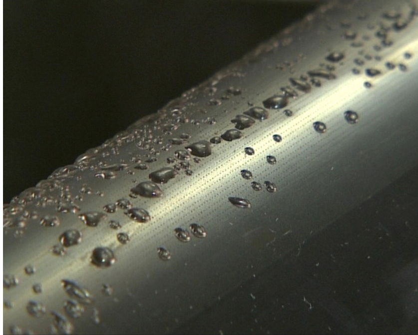
Figure 11. Weeping wing: glycol-based chemical fluid seeps through a mesh screen (TKS, 2012)
