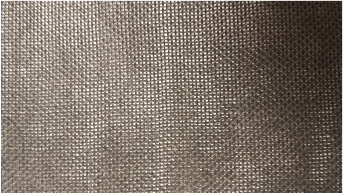
Figure 19. Mesh structure of carbon fabric
