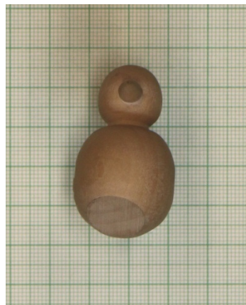
Figure B2. Wooden Bird with Chart Paper Background. The reference area was conveniently found in this way. The smallest squares are 1 \text{ mm}^2
