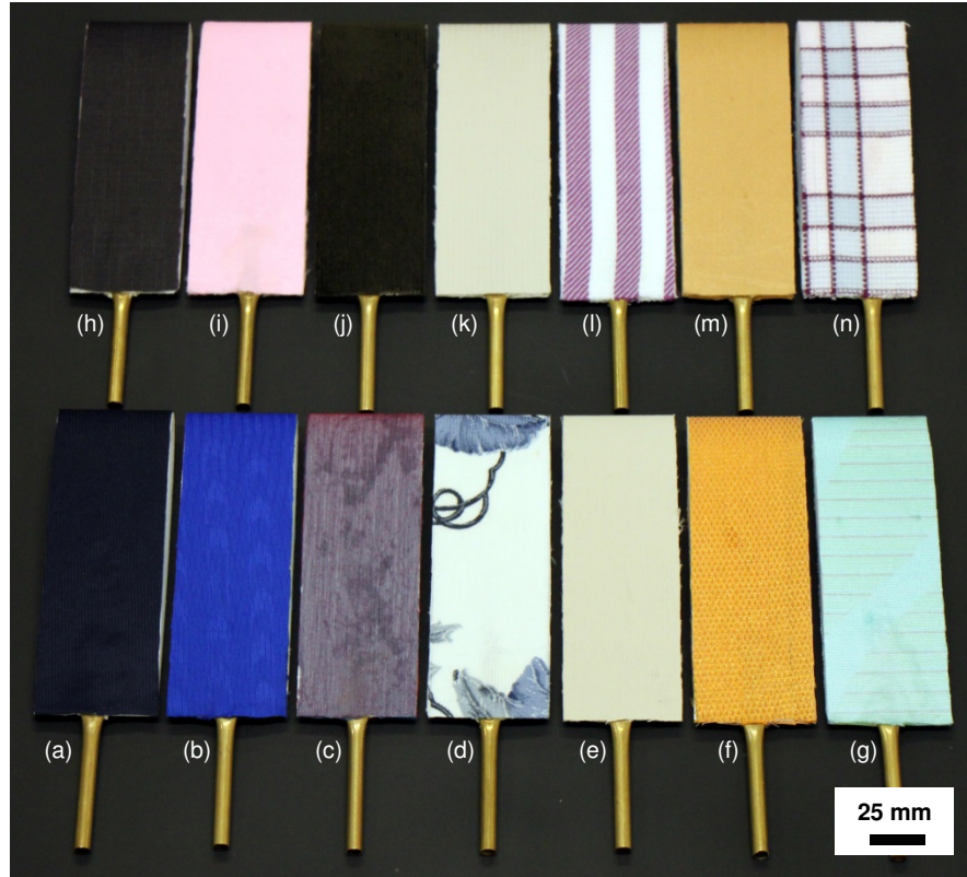
Figure 3.1. NACA 0012 Wing Models with Fabrics. (a) Navy Blue; (b) Fastskin ® FSI; (c) Purple; (d) Pattern; (e) Beige Thin; (f) Diamond; (g) Sky Blue; (h) Black; (i) Light Pink; (j) Corduroy; (k) Beige Thick; (l) Herringbone; (m) Gold; (n) Purple Stripe.
