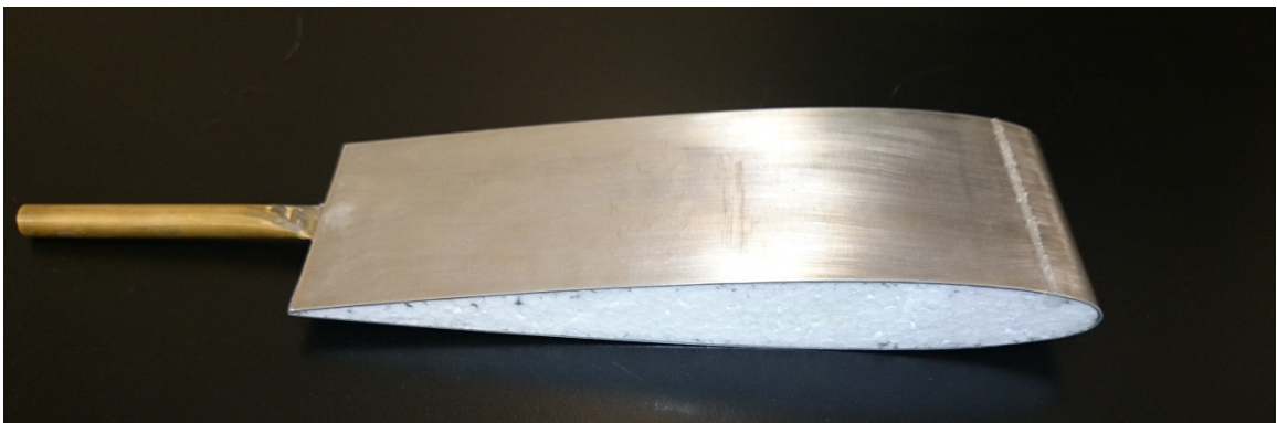
Figure 3.22a. Aluminum Wing Model with Boundary Layer Trip Strip (side view). For the wing model, the span is \sim 5.1 cm (2 in) and the chord is \sim 15.2 cm (6 in).
