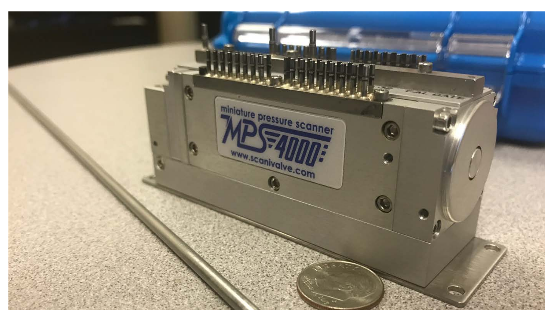
Figure 2: Scanivalve MPS 4000 Pressure Transducer
