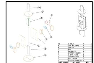
Figure 7. Nosecone Avionics
