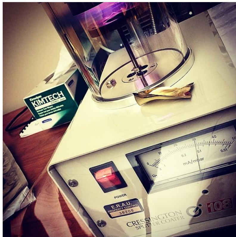
Figure 2.9 Sputter coating process.
