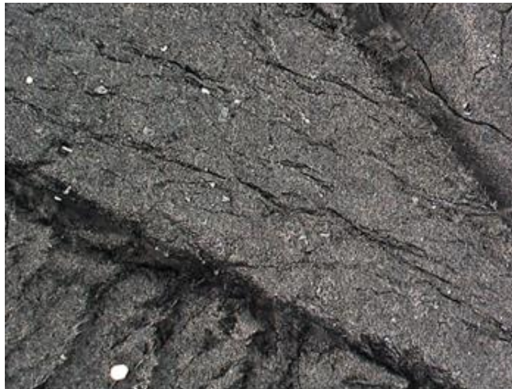
Figure 4.17 Surface image of overlapping layers due to delamination in Bucky paper IPMC.
