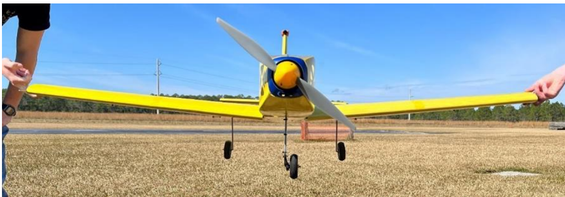
Figure 7-3: Wingtip load test
