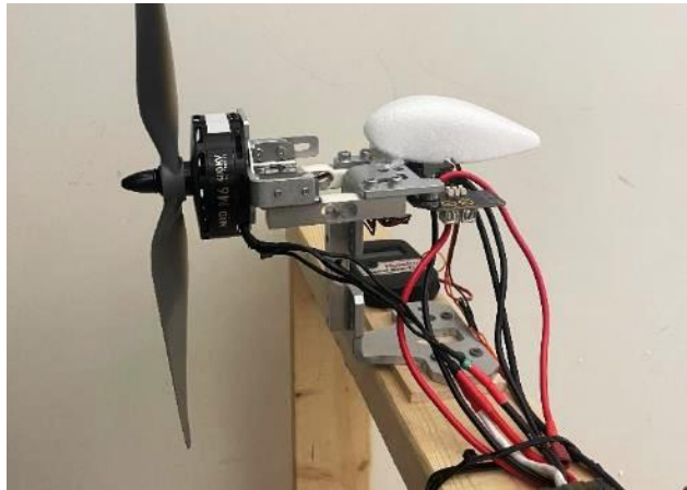
Figure 7-1: Static thrust test setup
