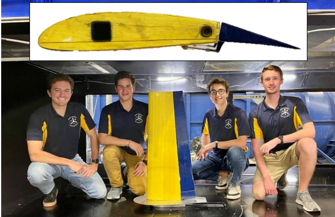
Figure 7-2: Full-scale wing model in the wind tunnel; SD7062 profile with 7.5-degree flap deflection (top)
