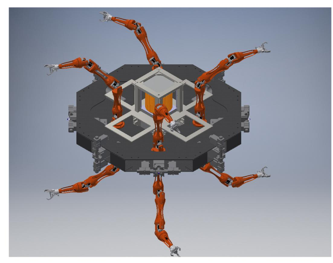
As seen in the photos above, the ARC prototype can be reconfigured to run with tools such as robotic arms, which could be used instead of EVA for spacecraft repair.
