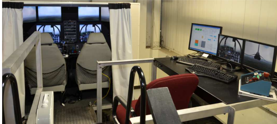
Figure 5.2 WVU Motion Based Simulator Interfaced with MATLAB/SIMULINK (Perez A. E., Moncayo, Perhinschi, Al Azzawi, & Togayev, 2015).
