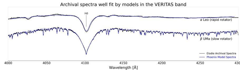
Figure 3: Model spectra from Equation [2] for  $\alpha$  Leo (top) and  $\beta$  UMa (bottom) compared to observed spectra. The rapid rotation of  $\alpha$  Leo broadens strong H $\delta$  line and washes out many of the weaker spectral lines seen in slow-rotator  $\beta$  UMa.
