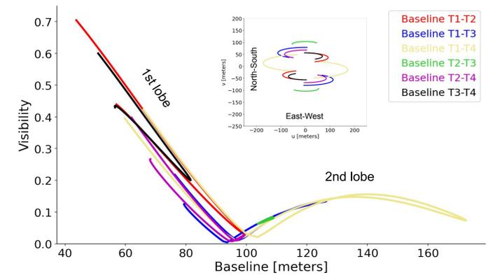
Figure 5: Model visibilities from Equation [1] for  $\alpha$  Leo are multi-valued in the 1st and 2nd lobes indicating rotational distortion. The T1-T3 visibilities are the lowest in the 1st lobe because they measure the wider equatorial axis ( $\sim$ North-South) of  $\alpha$  Leo, while the T1-T4 visibilities are among the highest in the 1st lobe because they measure along the narrower polar axis ( $\sim$ East-West) of  $\alpha$  Leo.
