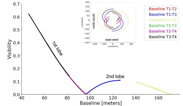
Figure 4: Model visibilities from Equation [1] for  $\beta$  UMa are single valued in the 1st and 2nd lobes indicating the star is circularly symmetric and not distorted. The T1-T3 and T1-T4 baselines have the highest resolution and sample the 2nd lobe.
