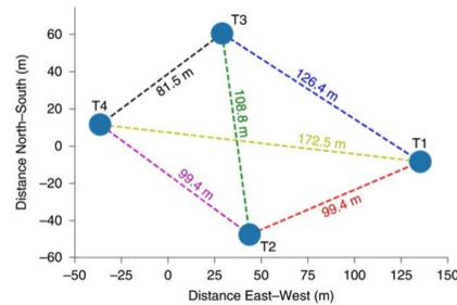
Figure 1: The Very Energetic Radiation Imaging Telescope Array System (VERITAS) is the first experiment to routinely perform Stellar Intensity Interferometry (SII) in the last 50 years. Six unique telescope pairs, yielding six interferometric baselines, can be formed using telescopes T1, T2, T3 and T4. Observations are made at 415 nanometers, in the blue.
