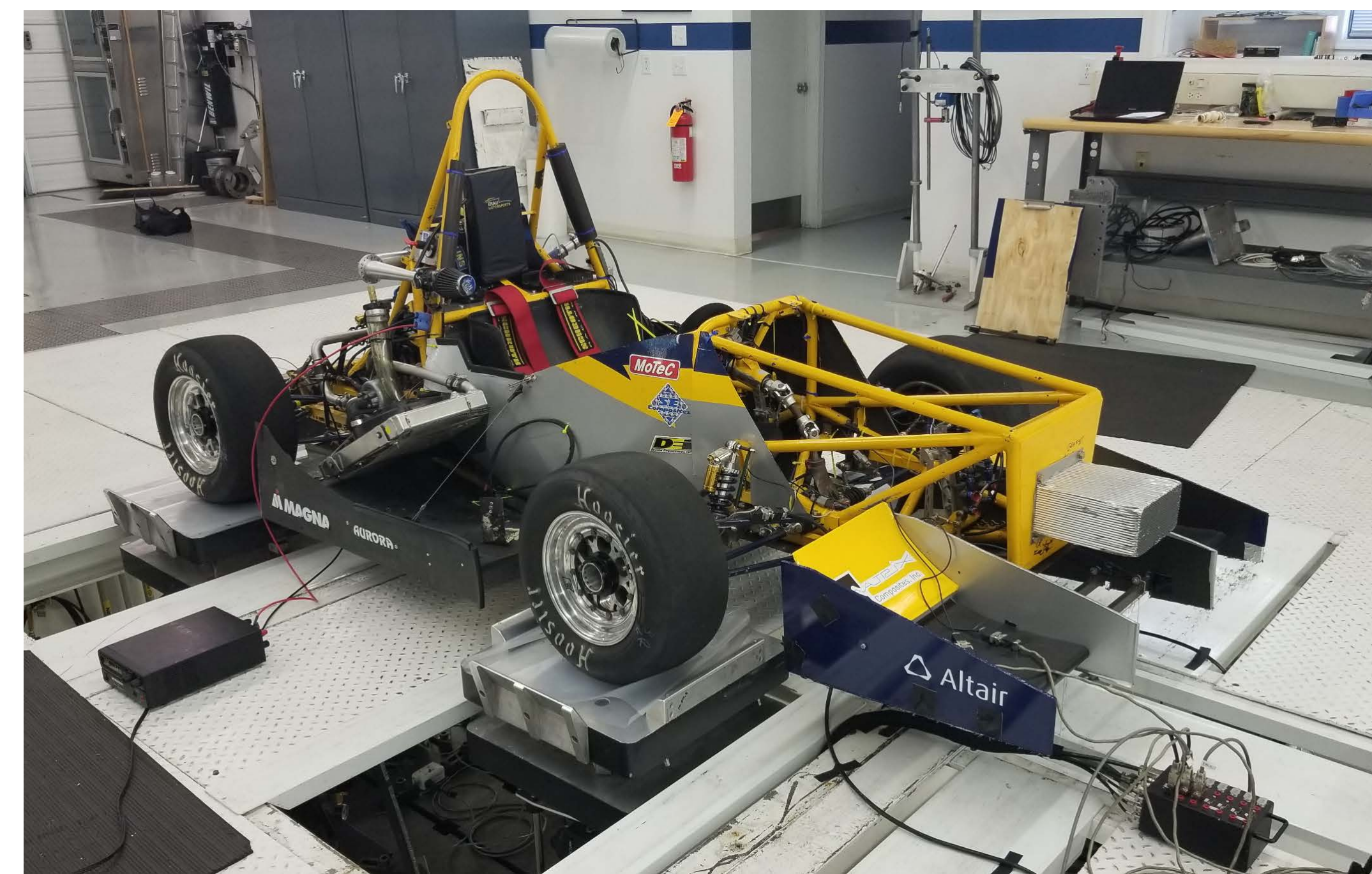
Figure 3: ER-03 on the OHLINS 4-Post Shaker Rig in Hendersonville, North Carolina
