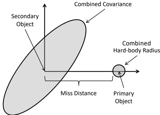
Figure 1: Conjunction-plane rendering of 2-D  $P_c$  calculation
