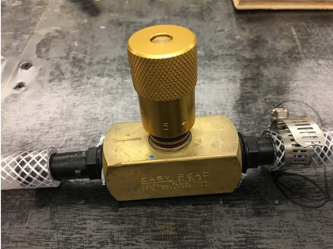
Figure 4.2: The figure showing the resistor installed in the MFL
