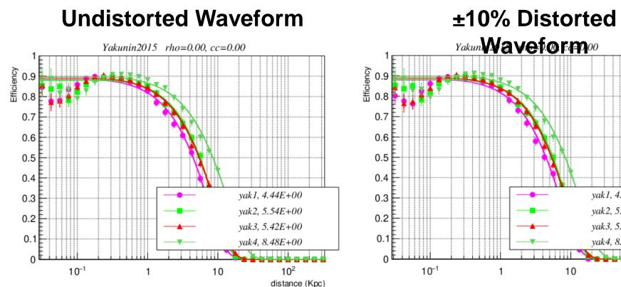
Above are preliminary results from the study, the plots denotes detection efficiencies as a function of distance, the first column pertains to a undistorted waveform, whereas in the second column, the same waveform was distorted using the  $\pm 10\%$  calibration error model.
