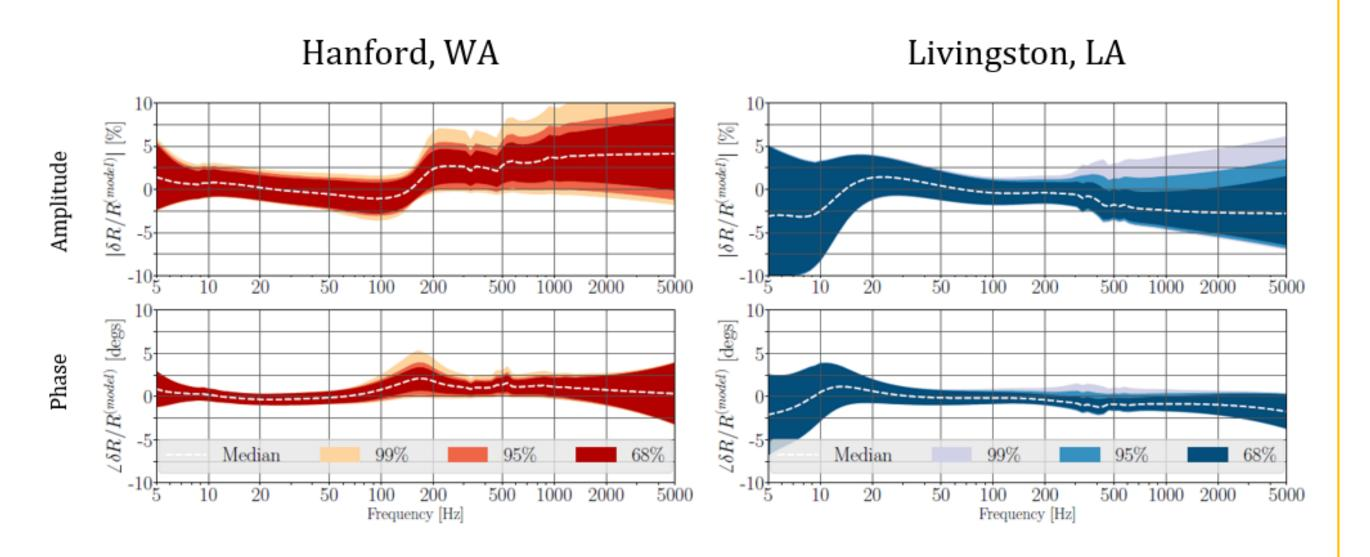
Calibration Uncertainties as a function of the frequency [Percentiles for Observing] Run Two. The percentiles are created for all of O2 data from November 30, 2016 to August 25th, 2017]
