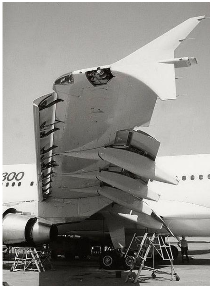
Figure 1. 10. Leading edge slats and flap deflection on an Airbus A310-300. Photo courtesy of Adrian Pingstone – Public Domain.
