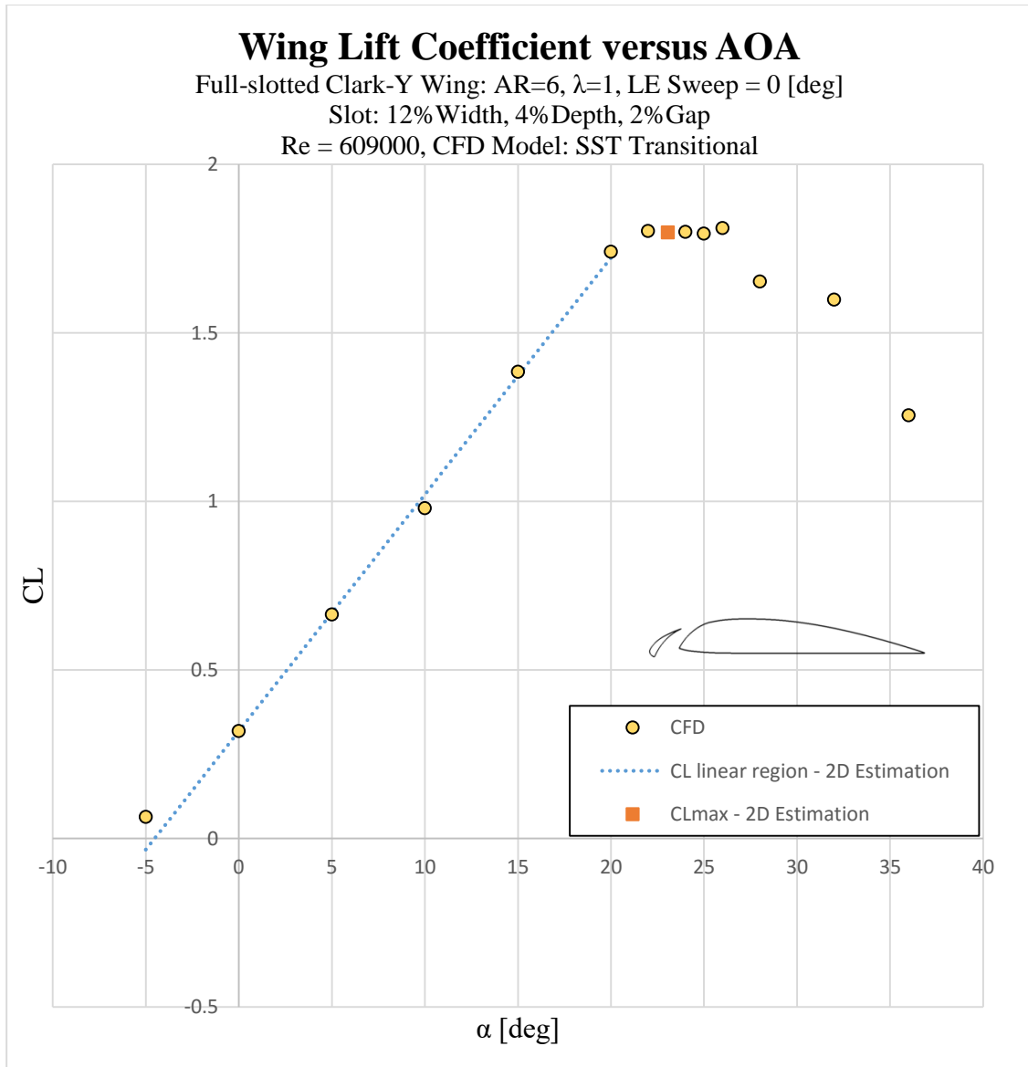
Figure 5. 4. Three-dimensional coefficient estimation for the full-slotted wing.
