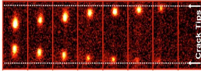
Figure 7. Infrared images of an internal crack. Adapted from “Acoustic Chaos for Enhanced Detectability of Cracks by Sonic Infrared Imaging,” by H. Xiaoyan et al., 2004, *Journal of Applied Physics*, 95(7), pp. 3792-3797.
