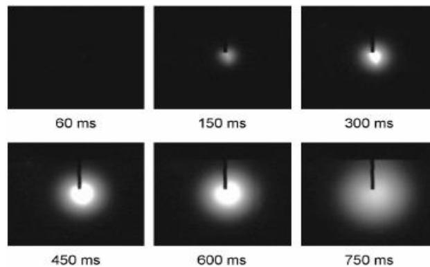
*Figure 6.* Infrared images taken at different excitation stages in an Aluminum bar with 1mm edge crack. Adapted from “Viscous Material-Filled Synthetic Defects for Vibrothermography,” by J. Renshaw, S. D. Holland, and D. J. Barnard, 2009, *NDT & E International*, 42(8), pp. 753-756.
