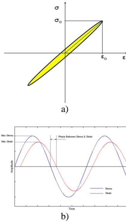
*Figure 1.* Hysteresis damping and energy dissipation in a material. A) Hysteresis loop and dissipated energy; b) Delay phase angle between stress and strain. Adapted from “FEM Modeling of Ultrasonic Vibrothermography of a Damaged Plate and Qualitative Study of Heating Mechanisms,” by A. S. Rizi, S. Hedayatrasa, X. Maldague, and T. Vukhanh, 2013, *Journal of Infrared Physics & Technology*, 61, pp. 101-110.
