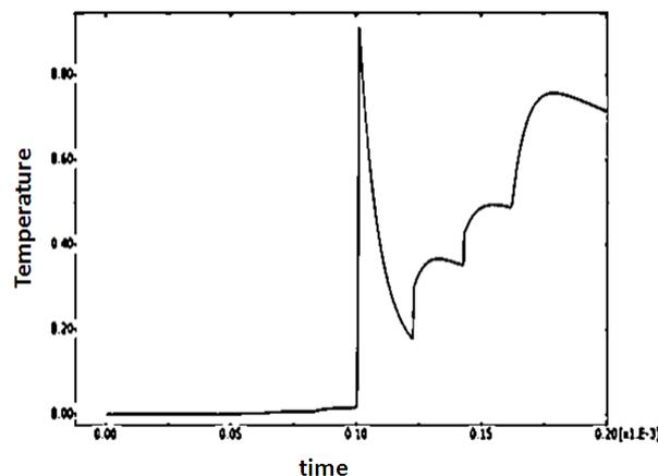
Figure 5. Temperature rise at edge crack tip versus time at 20 KHz excitation load.
