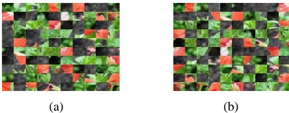
Figure 3 Processed Frame with Same N , but Different n and k . (a) Processed Frame with n=2 and k=14 , (b) with n=4 and k=23 .
