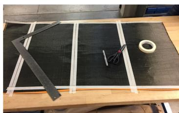
The plates were cut into 5"x6" samples.
