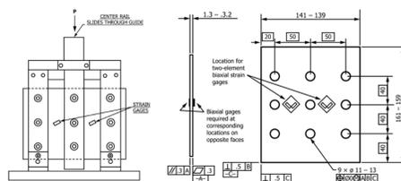
The 3 rail compression shear fixture
