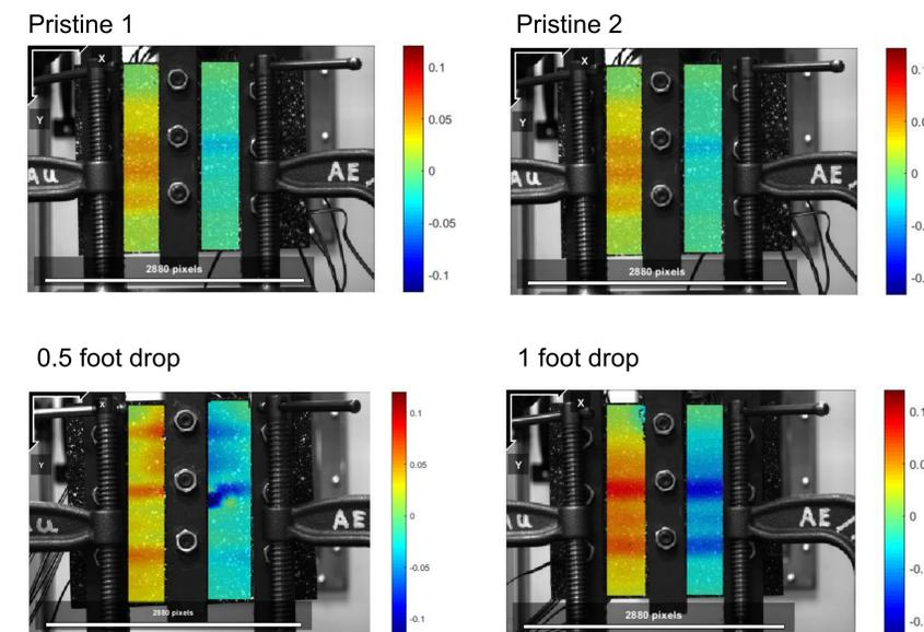
These images show the shear strain of each sample to the point of failure. The areas with warmer colors show high strain while areas with cooler colors show areas with relatively lower strain. As the magnitude of the impact increased, the amount of strain that each sample could withstand decreased. This is shown in the contrast of colors; the pristine samples have less color contrast than the damaged samples.
