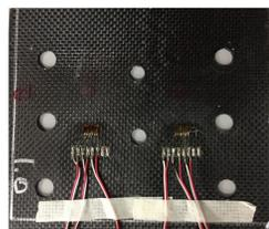
Strain Gauges were used to validate the DIC results.
