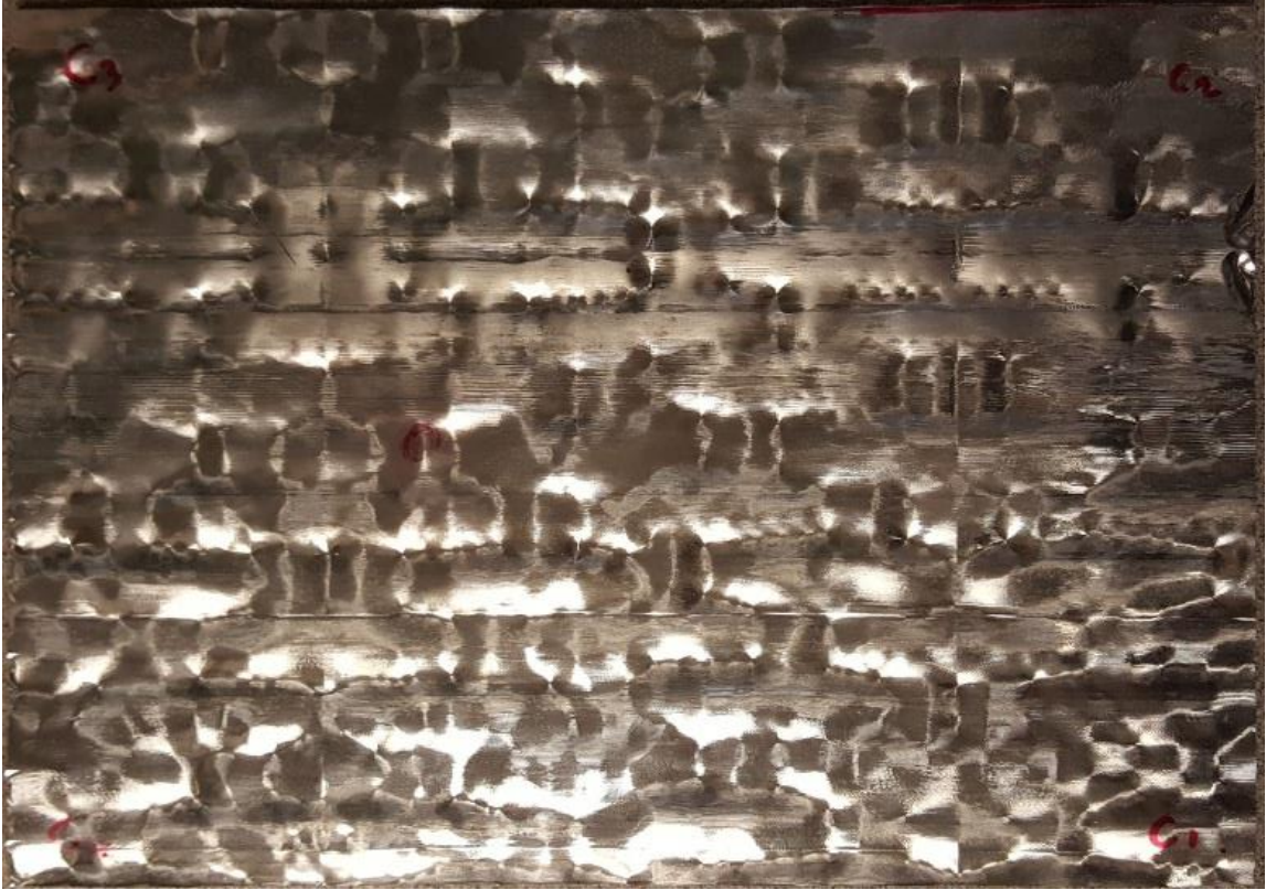
Figure 4.1: CNC machined CMC simulated surface
